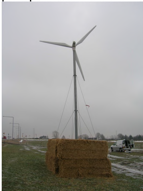
Figur 2. Photo taken in the direction of the turbine from the reference microphone position. Note the reference microphone is behind the bales of straw.
